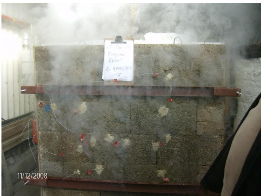
Exposed Surface After 4 Hours of Fire Testing
